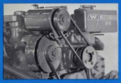
Standard 14 ampere generator mounted "piggyback" with extra 40 ampere alternator remains within basic outline of engine, readily accessible for service. It affords ample electricity for both engine starting and ships service.
