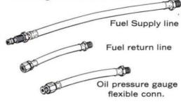
Flexible Hose Kit, available as an optional extra with your FOUR-107. Protects vulnerable fuel and lube oil pressure lines from vibration fatigue. Designed to fit exactly, these hoses protect your investment, prevent troublesome air leaks which sometimes result from careless plumbing, and reduce installation costs.
